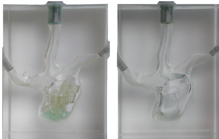
Fig. 2. Transparent silicone model of the aneurysm with and without coils.
