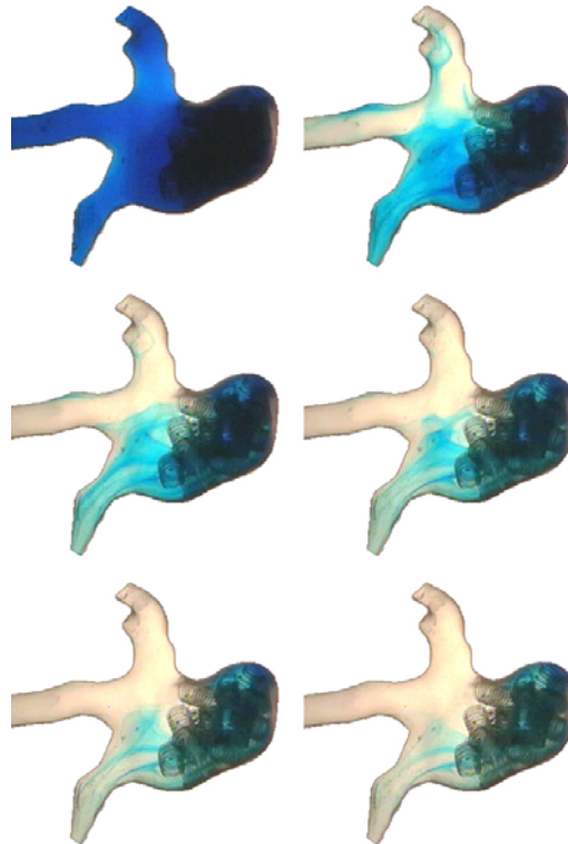
Fig. 4. Images of the dye washout in the aneurysm model filled with coils (15 % packing).
